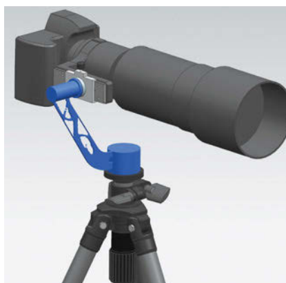
The optimization of a camera's mounting arm, completed in Siemens PLM Software's NX 8.5 with Topology Optimization.
