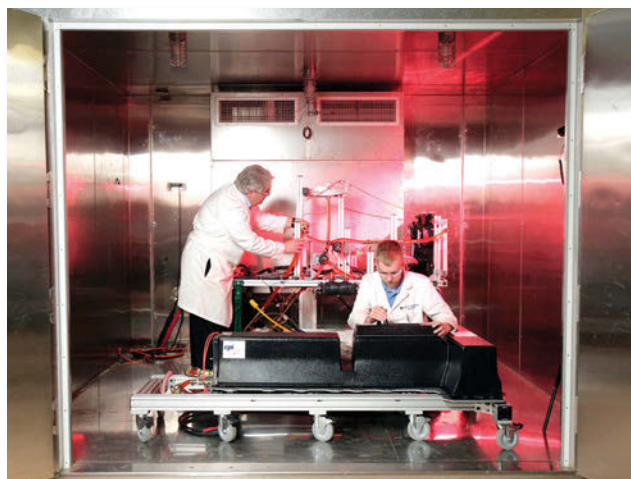
General Motors Battery Lab engineers prepare batteries for testing in the thermal chamber at the GM Tech Center in Warren, MI, in 2008. Photo by John F. Martin for General Motors.
