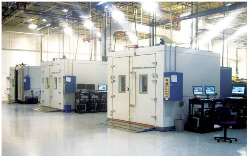
Intertek’s environmental chambers are used to prepare products before testing to meet requirements outlined in standards or test plans. Image courtesy of Intertek.
