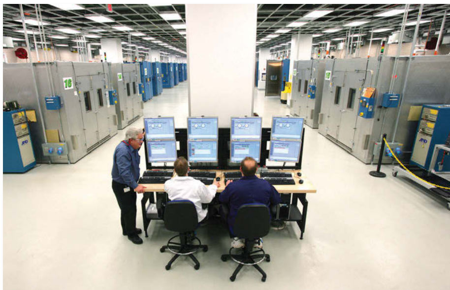
General Motors' 33,000 sq.-ft. Global Battery Systems Lab includes 160 test channels and 42 thermal chambers that duplicate extreme real-world driving patterns, hot and cold temperatures and calendar life. Photo by John F. Martin for General Motors.
